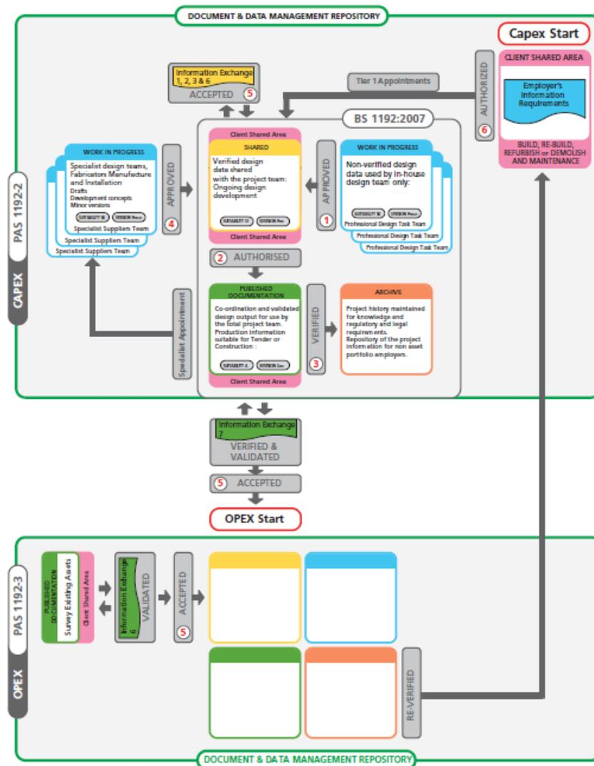
Figure 21 A Schematic of Common Data Environment (taken from PAS1192: Part 2)
