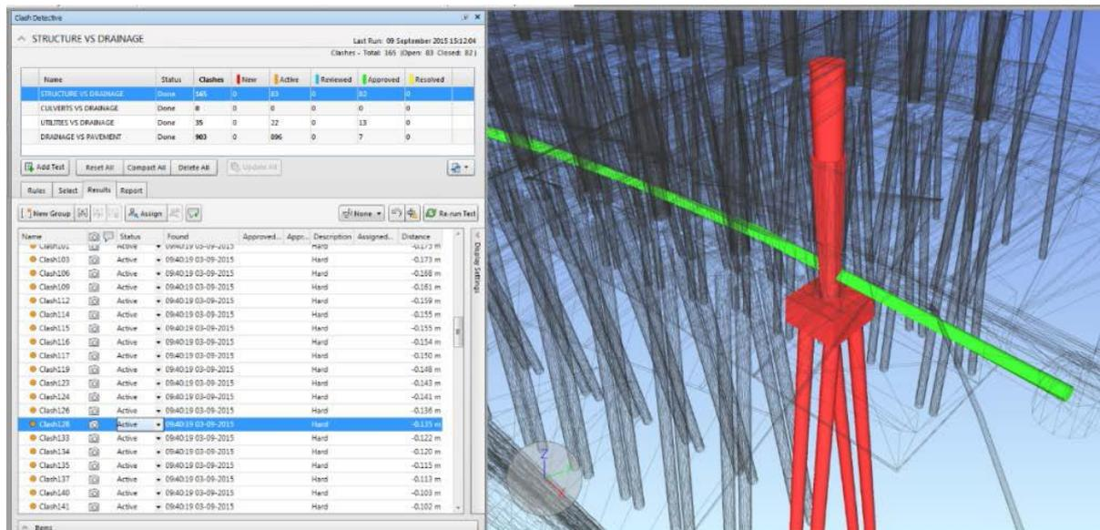
Figure 12 Risk Management and Clash Detection on the M8/M73/M74 Project
